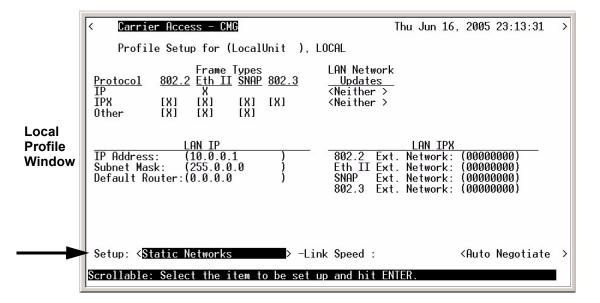
4. Select <IP Networks> or <Static IPX Networks>. Select [CTRL A] to add a Static Network.
